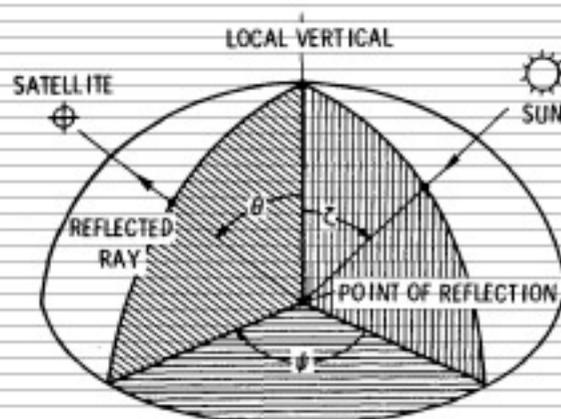
Fig. 4 Angular relationships for ERB measurements.
