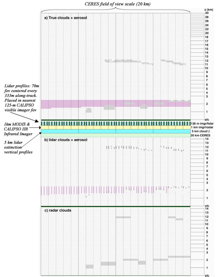
Figure 1. Schematic of a vertical profile aerosol and cloud layers for a) reference truth b) lidar sub-sampling with a 70m fov profile every 333m along the ground track, and c) radar with  $\sim 1$  km sampling along track.
